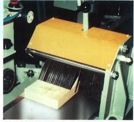
Anti-kickback Fingers (B23B or B29P) Special anti-kickback device for added safety when using slitting saw.
