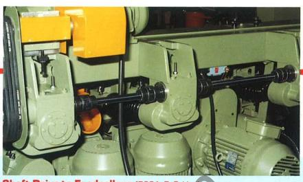
**Shaft Drive to Feedrollers** (B22A, B, G, H, J) Full Cardan shaft drive to feedrollers for reliable feed under continuous or heavy duty operation. Needs considerably reduced maintenance over chain drive.
