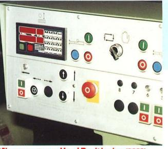
**Microprocessor Head Positioning** (B22S) Quick setting up by use of microprocessor memory units providing multi-programmable positioning of top and nearside heads.
